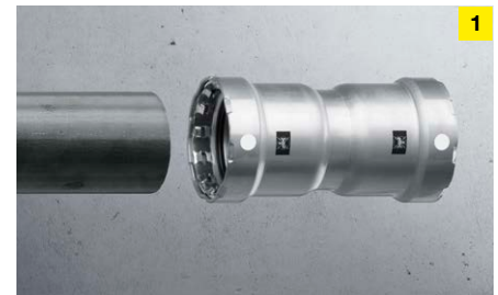
The steel pipe is cut to length and cleaned. Then the insertion depth is measured and marked, then the Megapress S connector is put on the pipe up to the mark.
