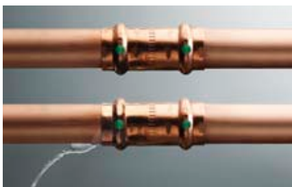
Above: sealed by pressing. Below: visibly unpressed.
