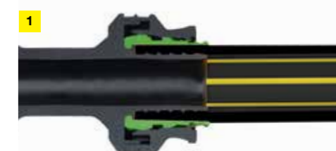
With the internal sealing contour of the Geopress K connector any other sealing element becomes obsolete.
